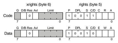
The **gray-shaded** bits are ignored in the value passed in. These are the Granularity and Limit, which are set by pmiSetLimit(). Regardless of the value passed, these bits of the descriptor are left untouched.
