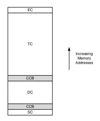
SC is the *start chunk*, EC is the *end chunk*, and CCB is a *chunk control block*. Until bins begin filling up due to smx\_HeapFree() operations, SBA-size chunks will come from DC, and larger chunks will come from TC. This results in small chunks being in lower heap and large chunks being in upper heap. This helps to reduce fragmentation caused by small, inuse chunks getting between larger free chunks, thus blocking them from being merged.
