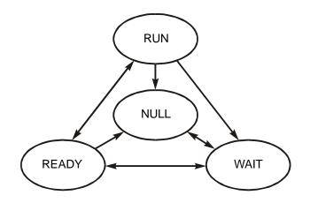
A task is in the NULL state prior to being created or after being deleted; it is in the WAIT state when it is waiting for an event such as receiving a message, a signal, or a timeout; it is in the READY state when it is ready to run; and it is in the RUN state when it is actually running. Only one task, at a time, may be in the RUN state, but any number of tasks may be in the other states. A task's state can be determined from the state field in its TCB.
