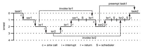
At time 0, task1 is running at nesting level 0. task1 makes an smx call which causes ssr1 to run at level 1. Before ssr1 can complete, it is interrupted by isr1, which runs at level 2 and invokes lsr1. Notice that lsr1 does not begin running immediately. Instead, it waits in the LSR queue, lq. isr1, itself, is then interrupted by isr2, which runs at level 3 and invokes lsr2. lsr2 is placed in lq after
