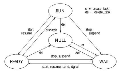
To help interpret the above diagram, remember that the task in the run state is the *current task*. By comparing this diagram to that for system services (see **task states** in Chapter 3 Introduction to Tasks), it is apparent that the only restriction on LSR calls is in causing the current task to leave the run state due to calling a *limited LSR* – see discussion, below.
