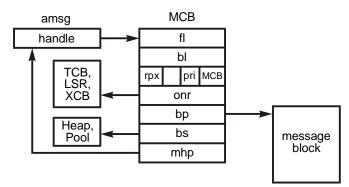
Note that an MCB has 28 bytes<sup>3</sup> vs. 16 bytes for a BCB. Hence, the overhead per message is higher, which tends to favor using smx blocks for small packets and smx messages for larger messages. However, in most cases, the benefits of exchange messaging overrule the overhead consideration — even for small packets.
