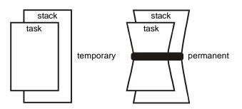
While running, there is no operational difference between one-shot tasks and normal tasks. Both can be preempted and both can be suspended to wait for events. Both retain their stacks, in these situations.
