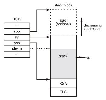
Note: Stacks grow "up" toward memory location 0. Hence "top" means the lowest address of the stack and "bottom" means the highest address of the stack. The stack pointer, sp, is predecremented on a push (write) and post-incremented on a pop (read).
