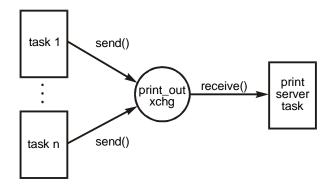
In this approach, a single server task is assigned to a resource. To access the resource, a client task prepares a message and sends it to an exchange, where the server task waits. Typically, the exchange is a pass exchange so the server runs at the message priority assigned by the client. The server task waits at the exchange for a message. When it receives a message, the server task accesses the resource and performs whatever is required by the message. For example:
