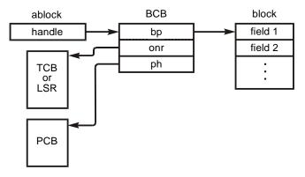
Note that the BCB is small — only 16 bytes. Hence, its overhead on a typical data block of 100 bytes size is small. This facilitates having hundreds of smx blocks in a system. However, if the BCB overhead is too great, then base blocks can be used instead.
