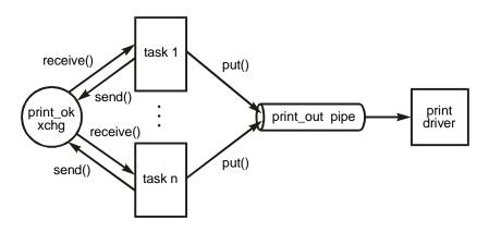
The use of exchanges for resource management involves assigning a token message per resource and an exchange to wait for a message. An advantage of this method is that the token message can contain information needed to use the resource — e.g. port number, speed, maximum packet size, type of error control, etc. The message can also accumulate usage information — e.g. number of sends, number of receives, average message length, average retries, etc.
