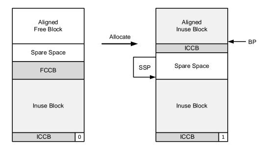
Aligned block allocations are enabled by EH\_ALIGN. Only power-of-two alignments are implemented. In order to prevent errors, the alignment parameter is the alignment number, **an**, as follows:
