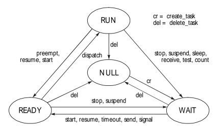
Except for preempt and dispatch, which are scheduler operations, and except for timeout, which is an LSR operation, each name represents a system service implemented by a system service routine (SSR). To interpret this diagram, it is helpful to realize that only the task in the run state (i.e. the current task) can call smx services. When the task is in another state, it cannot call
