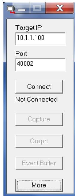
Enter the IP address of your target and click `Connect`. The message below the input box will change to `Connected` if it succeeds, and the `Capture` button will un-dim. Clicking `Capture` will cause it to read the event buffer from the target and then immediately open the event timelines window. The `Graph` and `Event Buffer` buttons open the event timelines and text event windows, respectively. These look the same as `smxAware GAT`. Each time `Capture` is clicked, the windows are updated.
